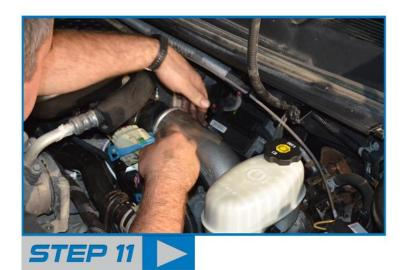
Now you have to get the tube into the boot at the turbo charger. This will be a bit more difficult than the factory hot side due to the upgraded boots. It is easiest to push the tube down on the boot and gently working the boot over the tube using a hose pick or a blunt end screw driver.
