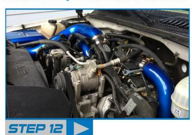
With the hot side in place make sure there is plenty of room between the hot side and brake booster. Now tighten the other two clamps and reinstall the wheel well.
