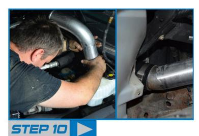
Slide the new hot side intercooler tube in to position being careful not to scratch it. With it in place slide it all the way into the boot at the intercooler.
