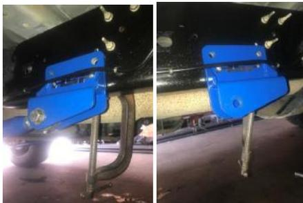
11. You must now drill ½" holes in the frame using a ½" drill bit. It is best to drill one hole at a time and install the bolt and washers after each hole and torque to 30 ft-lbs. Use a ½" drill bit first to mark a center hole then drill through with a 3/8" drill bit. After the 3/8" hole is drilled then use the ½" bit to open the hole up the rest of the way.
