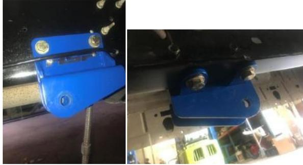
12. With all 4 holes drilled re-torque the ½” bolts to 30 ft-lbs.
