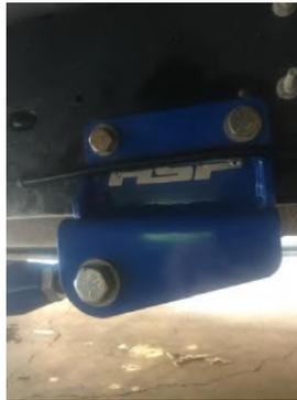
13. With the brackets in place torque the front 5/8” bolts to 50 ftlbs.
